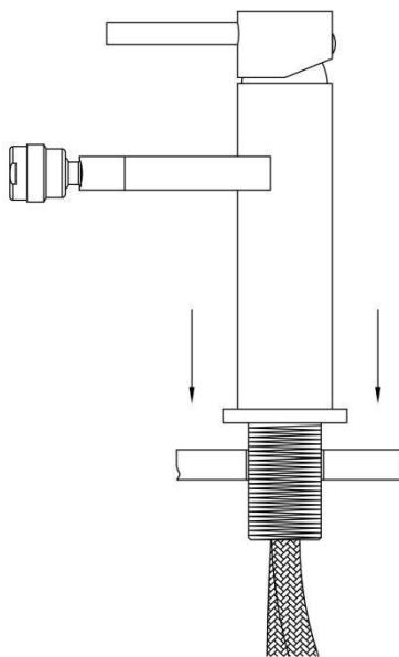
3. Install the bottom gasket and mounting washer on the threaded mounting tube.
