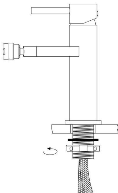
4. Tighten the gasket on the threaded mounting tube. Align and tighten the faucet. Carefully check the installation and tightness of the faucet.
