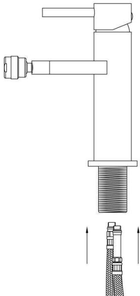
2. Then, insert the flexible connection hoses and threaded mounting tube into the hole on the bidet. Before performing this operation, make sure that the seal in the faucet base is in its place.
